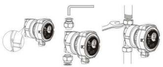
4.2. The pump should be installed in such a way that the pump shaft is horizontal.
